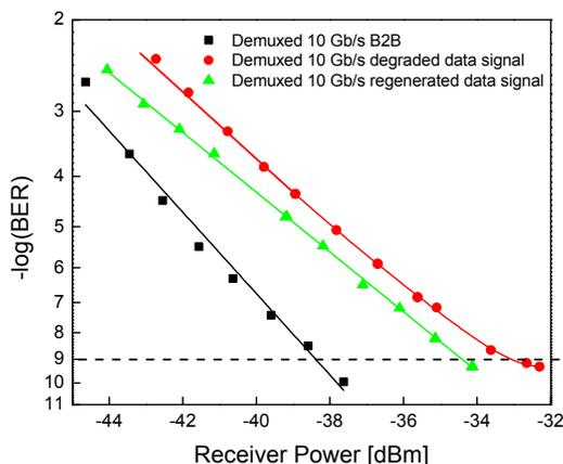
Figure 3. BER performance of the silicon nanowire based regenerator. A 2 dB improvement of the receiver power is achieved at  $10^{-9}$ .
