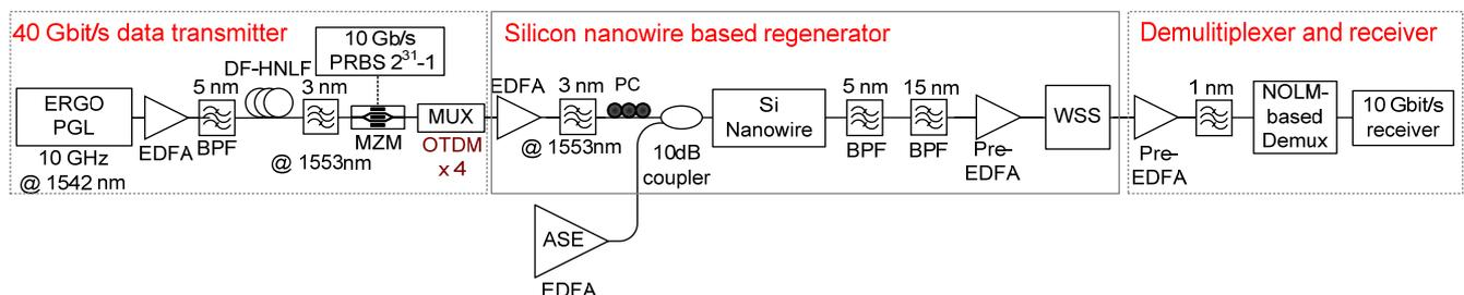
Figure 1. Experimental setup of silicon nanowire based all-optical signal regeneration.
