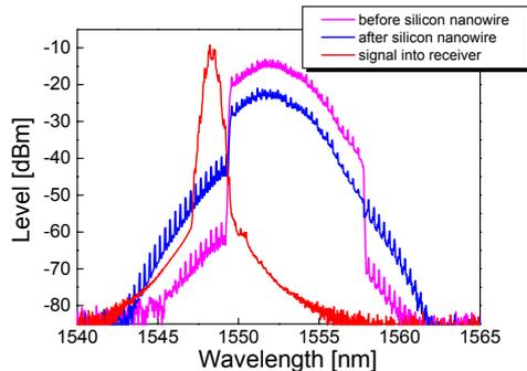
Figure 2. Optical spectra of the 40 Gbit/s data signal, measured before and after the silicon nanowire and before the demultiplexer.
