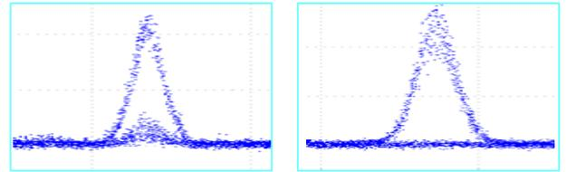
Figure 4. Eye-diagrams. (left) degraded data signal. (right) regenerated data signal.
